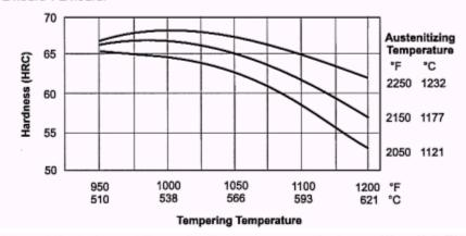
Effect of Hardening and Tempering Temperatures on Hardenss—Micro-Melt T15 Alloy All samples were austenitized in salt for the indicated time at the indicated temperature, oil quenched, and tempered at the indicated temperature for 2 hours + 2 hours.
