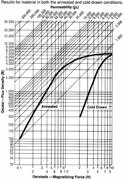
DC Magnetization Permeability Curves - Free-Cut Invar "36" Alloy Results for material in both the annealed and cold drawn conditions.
