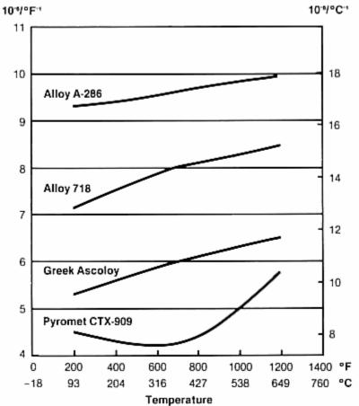
Mean coefficient of thermal expansion
