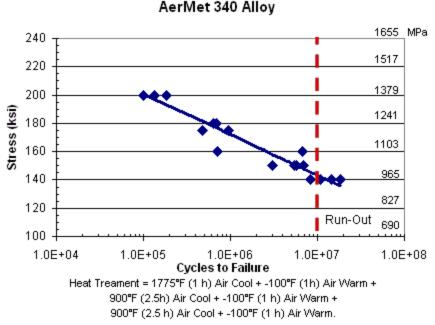
Rotating Bending (R = -1, Kt = 1) Fatigue Life of AerMet 340 Alloy
