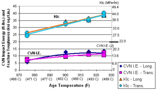
Heat Treatment = 1775°F (968°C) (1 h) Air Cool + -100°F (-73°C) (1 h) Air Warm + 875°, 900°, 915° or 925°F (468, 482, 491 or 496°C) (2.5 h) Air Cool + -100°F (-73°C) (1 h) Air Warm + 875°, 900°, 915° or 925°F (468, 482, 491 or 496°C) (2.5 h) Air Cool + -100°F (-73°C) (1 h) Air Warm.
