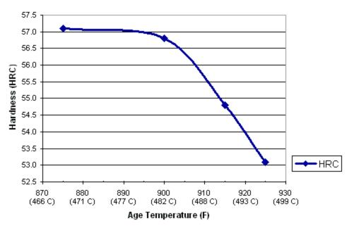
Heat Treatment = 1775°F (968°C) (1 h) Air Cool + -100°F (-73°C) (1 h) Air Warm + 875°, 900°, 915° or 925°F (468, 482, 491 or 496°C) (2.5 h) Air Cool + -100°F (-73°C) (1 h) Air Warm + 875°, 900°, 915° or 925°F (468, 482, 491 or 496°C) (2.5 h) Air Cool + -100°F (-73°C) (1 h) Air Warm.
