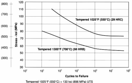
Tempered 1025°F (550°C) = 130 ksi (896 MPa) UTS Tempered 1300°F (700°C) = 103 ksi (710 MPa) UTS
